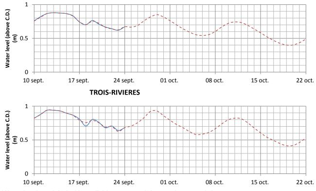
\* Water level modeled with available measured data and expected data
