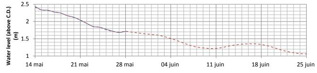
\* Water level modeled with available measured data and expected data
